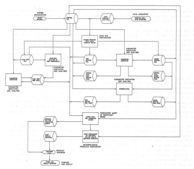
Figure 1. Wind profiler software flow chart diagram indicating the software processes and data files accessed for each step in the system.
