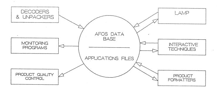
Figure 1. Components of the TDL Local Applications System.
