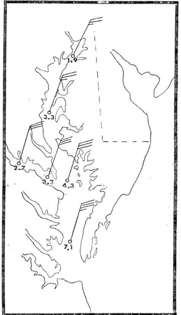
Figure 5. Twelve-hour forecasts of wind and waves valid at 1200 GMT on October 25, 1982. Wind forecasts are 1000-mb LFM winds interpolated to the wave forecast points.
