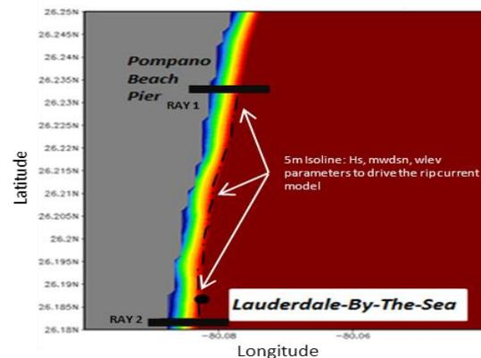
**Figure 3.** A set of rays built within the Fort Lauderdale NWPS grid that intersects the desired 5m bathymetric contour. Wave output along this contour is used as input to force the rip current model.
