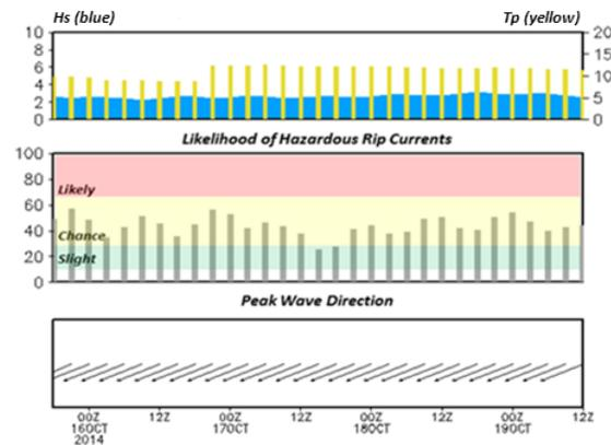
**Figure 5.** Three panel time series highlighting the total significant wave heights and periods (top panel), likelihood of rip currents (middle panel), and wave direction (bottom panel).
