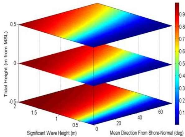
**Figure 4.** 3D graphical depiction of the rip current model that outputs the likelihood of hazardous rip currents from 0 to 1 based on: total significant wave height (y), mean wave direction (x) and water level (z).
