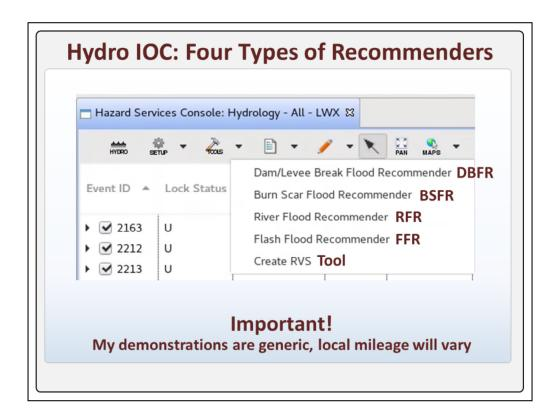
There are four types of recommenders and one tool in hydro IOC. The recommenders include: **dam/levee** break flood, **burn** scar flood, **river** flood, and **flash** flood. The single tool in IOC is the **Create** RVS tool. Recommenders tend to provide initial hazard events for the HID while Hazard Services tools are more generic and do not assemble hazard events for the HID.
