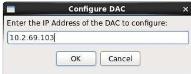
Exhibit 32.6-5 Enter the address of the spare DAC
