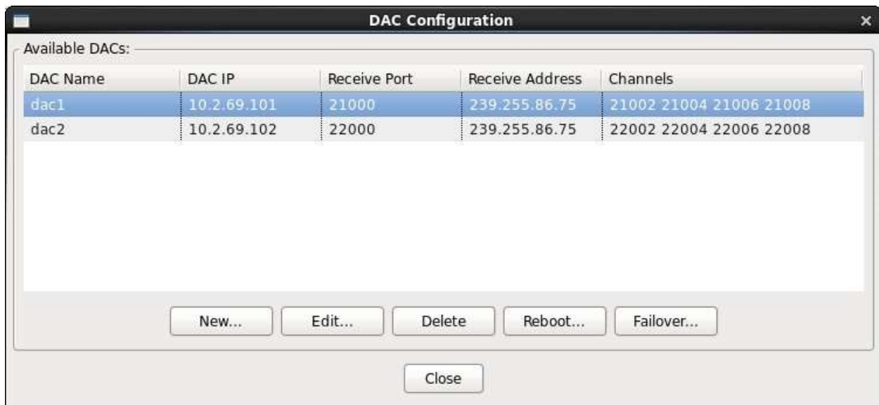
Exhibit 32.6-8 DAC Configuration screen after failover
