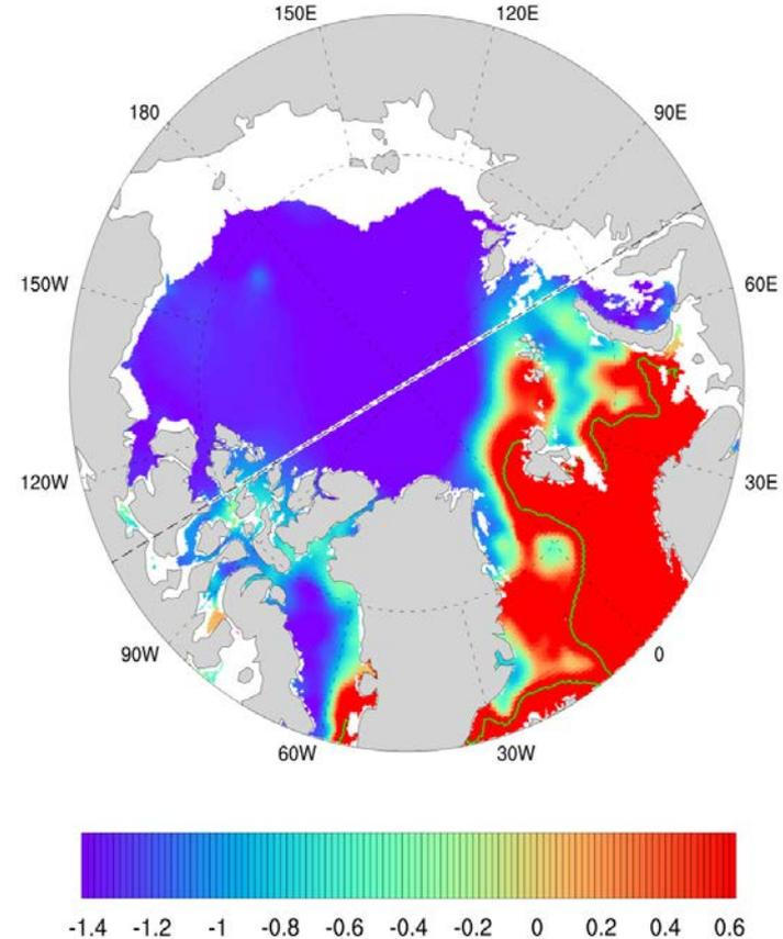
At 100m, MOM6 initialized from CFSRv2 exhibits both artifacts from the tripolar grid (seam) and an unrealistically strong inflow at Bering Strait. The Eurasian shelves and Bering Strait are too deep. There is a weak Atlantic inflow signal with primarily recirculation at Fram Strait, as indicated by the 1.8 °C contour line shown in green.
