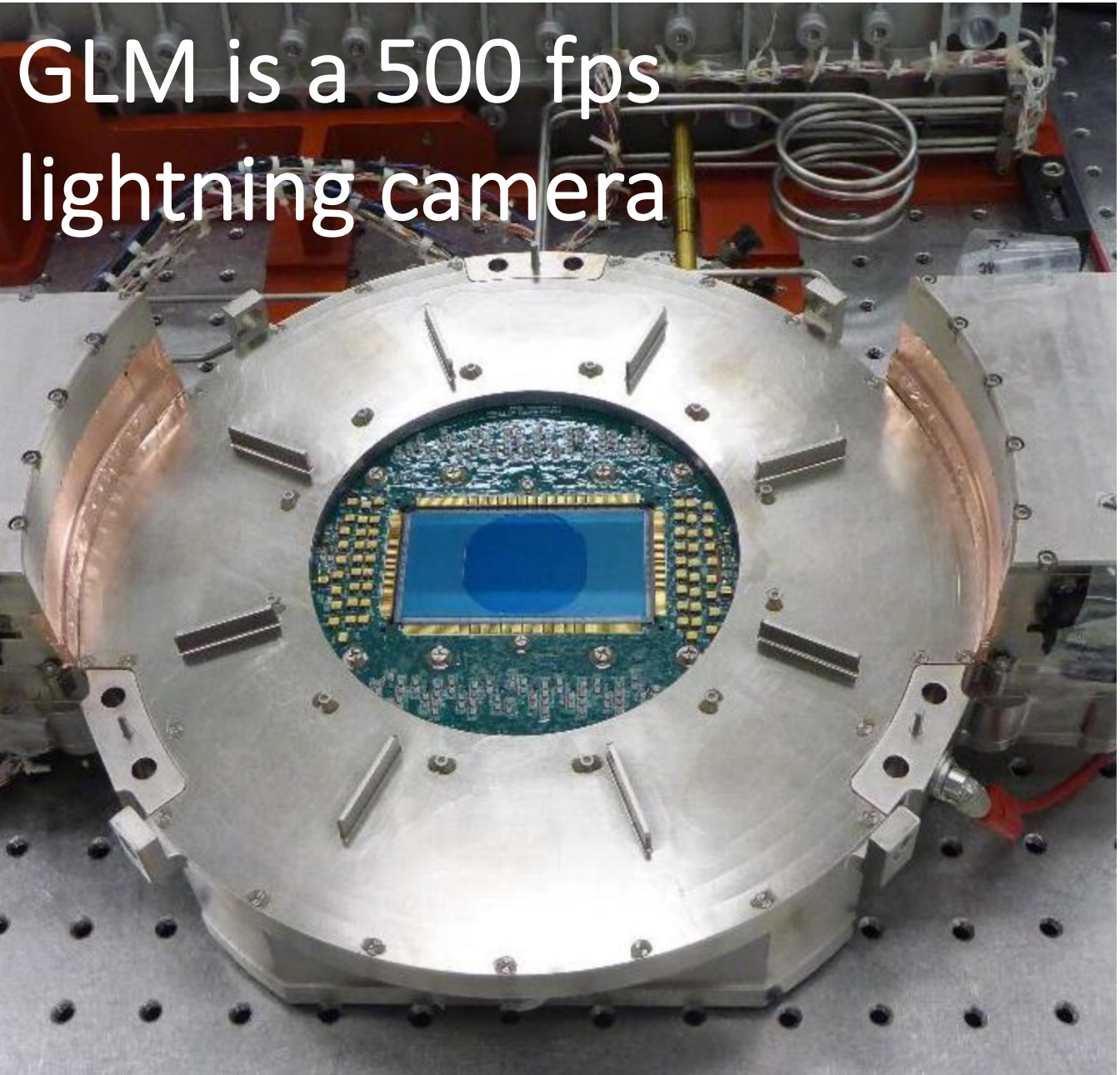
On-board processing reduces raw video by a factor of > 1000x
