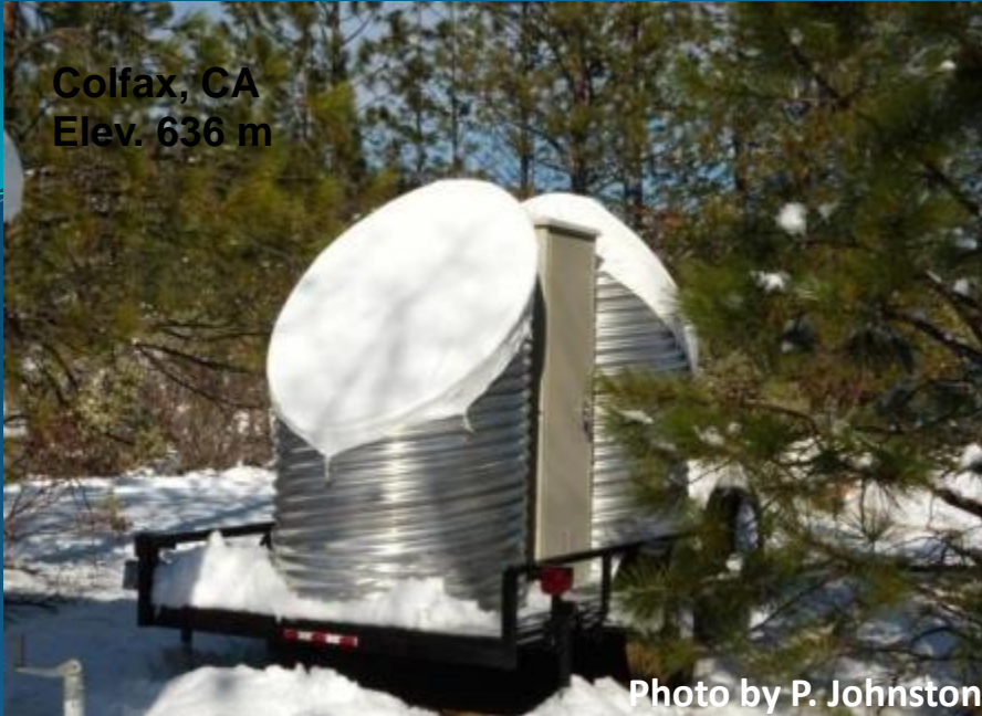
ESRL Physical Sciences Division FMCW S-band Snow Level Radar
