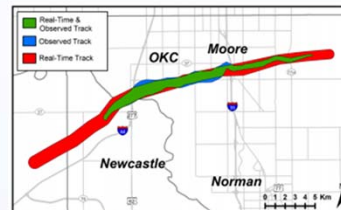
Figure 4. Example of the object-based geospatial verification technique developed to evaluate the quality of the proposed damage paths of this study. Green areas correspond to hits, blue areas are misses, and red areas are false detections. An electronic supplement for analyzing the classification method of geospatial verification for each damage path is available at hvt.nssl.noaa.gov/damagepaths/verification.php .
